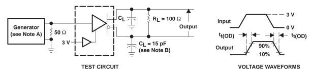
NOTES: A. The input pulse is supplied by a generator having the following characteristics:  $t_f \le 5$  ns,  $t_f \le 5$  ns, PRR  $\le 1$  MHz, duty cycle = 50%,  $Z_{\Omega} = 50 \ \Omega$ .
