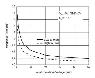
Fig. 8 Response Time vs. Input Overdrive Voltage
