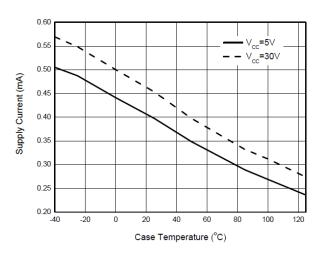
Fig. 2 Supply Current vs. Case Temperature
