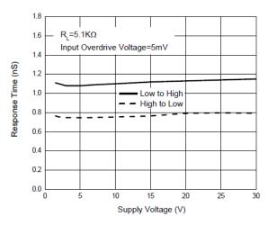
Fig. 9 Response Time vs. Supply Voltage
