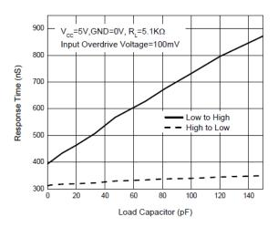
Fig. 7 Response Time vs. Load Capacitor
