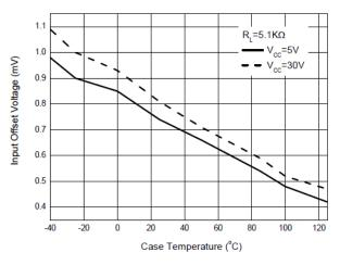
Fig. 3 Input Offset Voltage vs. Case Temperature
