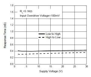
Fig. 10 Response Time vs. Supply Voltage
