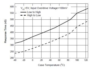
Fig. 6 Response Time vs. Case Temperature
