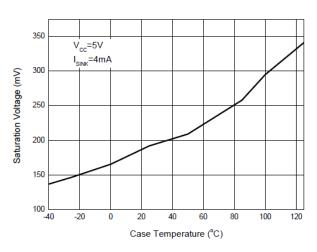
Fig. 4 Saturation Voltage vs. Case Temperature
