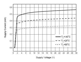
Fig. 1 Supply Current vs. Supply Voltage
