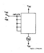
Fig. 11 - Quiescent-device-current test circuit.
