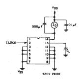
Fig. 14 - Dynamic power dissipation test circuit.
