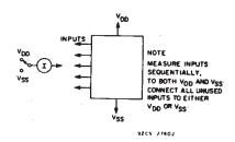
Fig. 12 - Input current test circuit.
