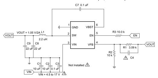
Figure 8-1. TPS562201 and TPS562208 1.05-V/2-A Reference Design
