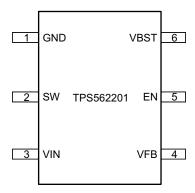
Figure 5-1. 6-Pin SOT DDC Package (Top View)
