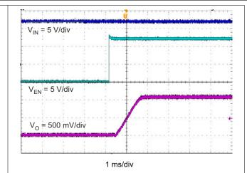
Figure 8-14. TPS562201 Start-Up Relative to  $V_{\text{I}}$
