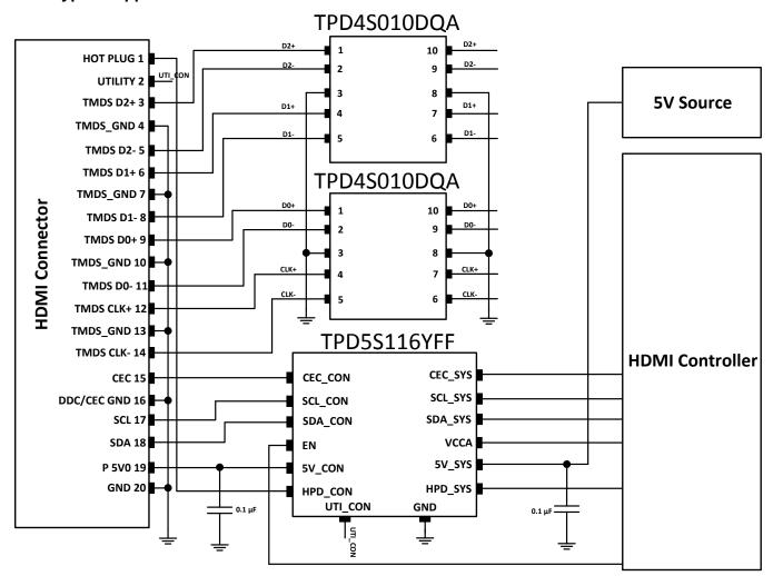
Figure 8. Typical Application Schematic
