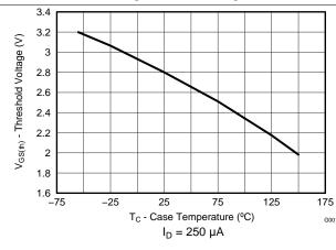
Figure 6. Threshold Voltage vs Temperature
