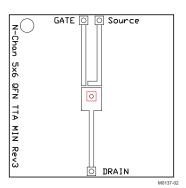
Max  $R_{\theta JA} = 115^{\circ} C/W$  when mounted on a minimum pad area of 2-oz. (0.071-mm thick) Cu.
