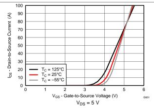
Figure 2. Saturation Characteristics
