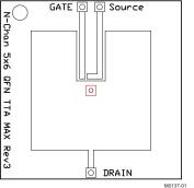
Max  $R_{\theta JA} = 50^{\circ} C/W$  when mounted on 1 inch² (6.45 cm²) of 2-oz. (0.071-mm thick) Cu.
