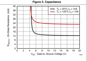
Figure 7. On-State Resistance vs Gate-to-Source Voltage
