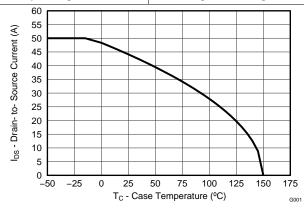
Figure 12. Maximum Drain Current vs Temperature
