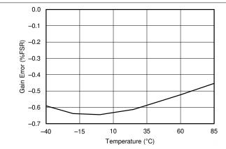
Figure 7-4. Coulomb Counter Gain Error (from –0.2 V to 0.2 V)
