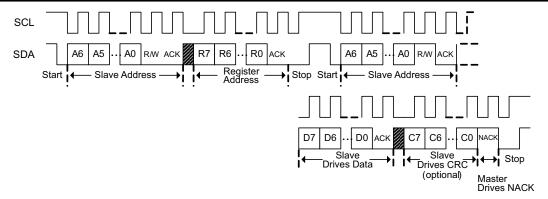
Figure 8-5. I<sup>2</sup>C Read Without Repeated Start
