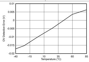
Figure 7-6. OV Protection Detection Error (0xFF Setting)
