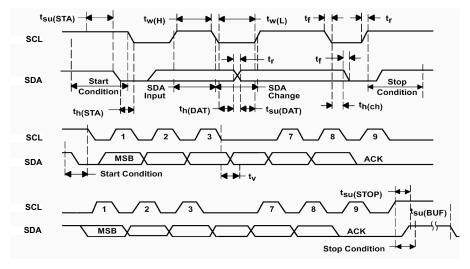
Figure 7-1. I<sup>2</sup>C Timing
