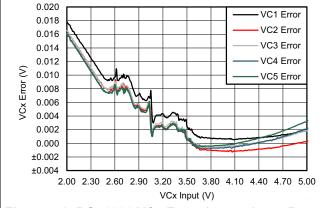
Figure 7-2. BQ76930 VCx Error Across Input Range at 25°C with VIN at 3.6 V
