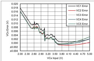
Figure 9-5. BQ76930 VCx Error Across Input Range at 25°C
