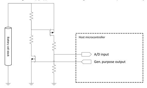
Figure 8-1. External Real-Time Calibration Circuit to Host Microcontroller
