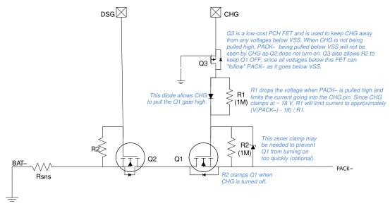
Figure 8-2. CHG and DSG FET Circuit
