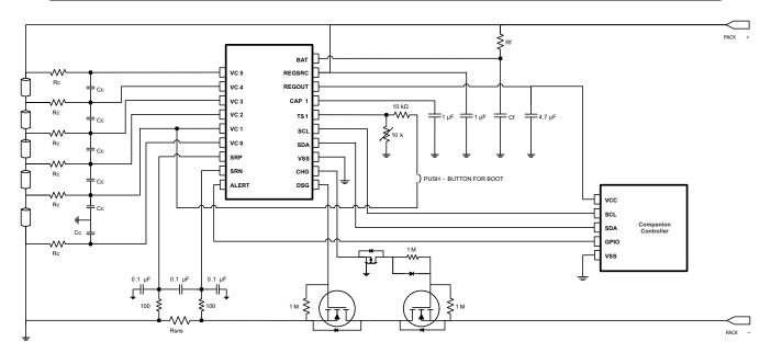
Figure 9-1. BQ76920 with BQ78350 Companion Controller IC
