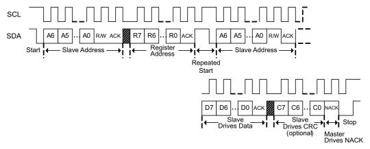
Figure 8-4. I<sup>2</sup>C Read with Repeated Start
