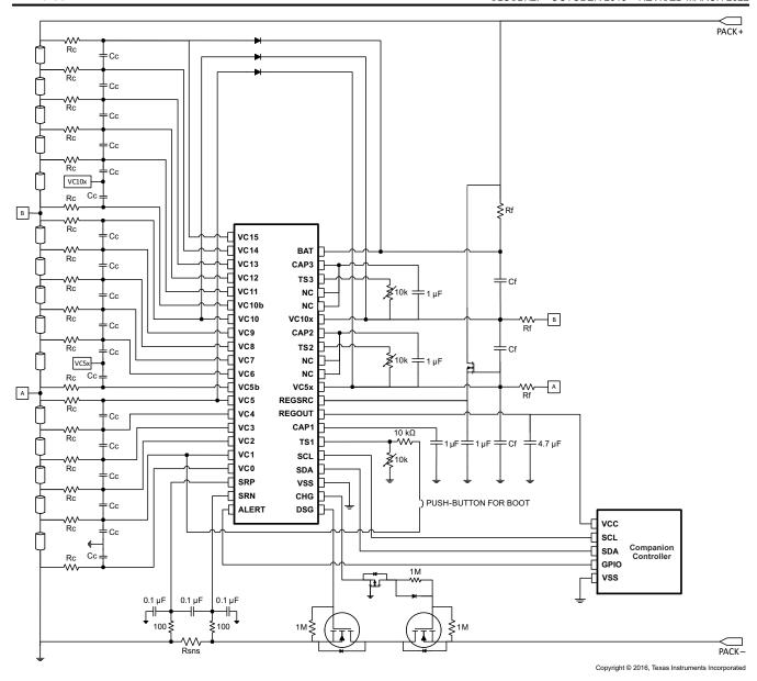
Figure 9-3. BQ76940 with BQ78350 Companion Controller IC
