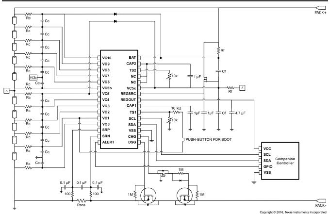
Figure 9-2. BQ76930 With BQ78350 Companion Controller IC
