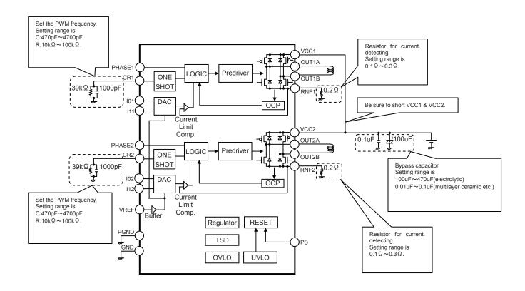
Fig.1 Block diagram & Application circuit diagram
