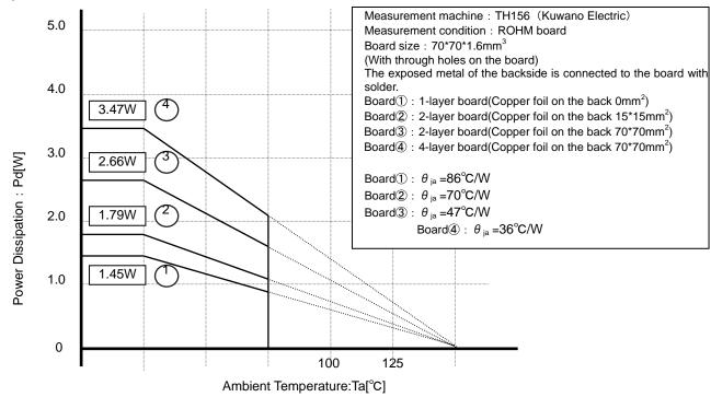
Fig. 2 HSOP25 Derating curve
