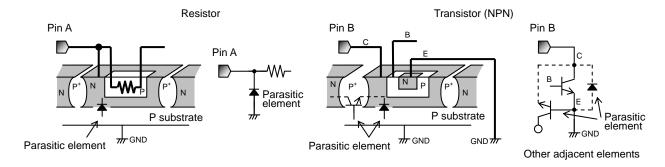
Fig.3 Pattern Diagram of Parasitic Element
