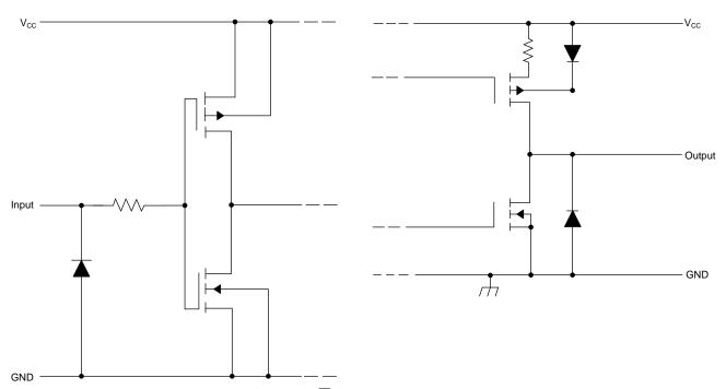
Figure 8. Equivalent of Each Input (A, G, or  $\overline{G}$ ) Schematic
