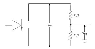
Figure 3. Test Circuit,  $V_{\text{OD}}$  and  $V_{\text{OC}}$
