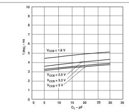
Load Capacitance T<sub>A</sub> = 25°C, V<sub>CCA</sub> = 2.5 V
