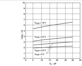
Figure 6-13. Typical Propagation Delay of High-to-Low (A to B) vs Load Capacitance  $T_A = 25^{\circ}C$ ,  $V_{CCA} = 5 \text{ V}$
