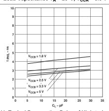
Figure 6-11. Typical Propagation Delay of High-to-Low (B to A) vs Load Capacitance T<sub>A</sub> = 25°C, V<sub>CCA</sub> = 3.3 V
