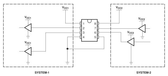
Figure 9-1. Unidirectional Logic Level-Shifting Application
