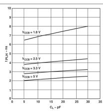
Figure 6-14. Typical Propagation Delay of Low-to-High (A to B) vs Load Capacitance  $T_A = 25$ °C,  $V_{CCA} = 5$  V
