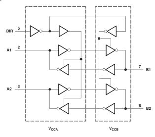
Figure 8-1. Logic Diagram (Positive Logic)
