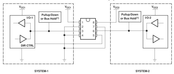
Figure 9-2. Bidirectional Logic Level-Shifting Application
