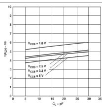
Figure 6-7. Typical Propagation Delay of High-to-Low (B to A) vs | Figure 6-8. Typical Propagation Delay of Low-to-High (B to A) vs Load Capacitance T<sub>A</sub> = 25°C, V<sub>CCA</sub> = 2.5 V
