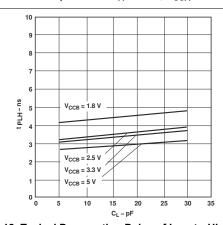
Figure 6-12. Typical Propagation Delay of Low-to-High (B to A) vs Load Capacitance  $T_A = 25$ °C,  $V_{CCA} = 3.3 \text{ V}$
