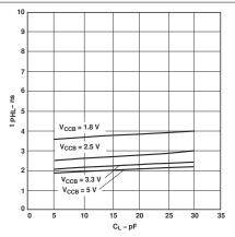
Figure 6-15. Typical Propagation Delay of High-to-Low (B to A) vs Load Capacitance T<sub>A</sub> = 25°C, V<sub>CCA</sub> = 5 V
