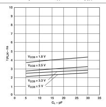
Figure 6-16. Typical Propagation Delay of Low-to-High (B to A) vs Load Capacitance  $T_A = 25^{\circ}C$ ,  $V_{CCA} = 5$  V
