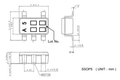
Fig.30 External Dimensions of BH7673G Package
