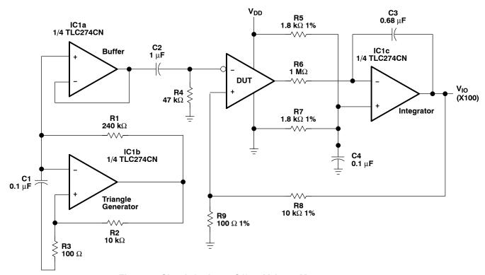
Figure 6. Circuit for Input Offset Voltage Measurement
