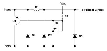
Figure 1. LinCMOS™ ESD-Protection Schematic
