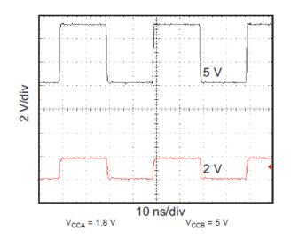
Figure 12. Level-Translation of a 2.5-MHz Signal
