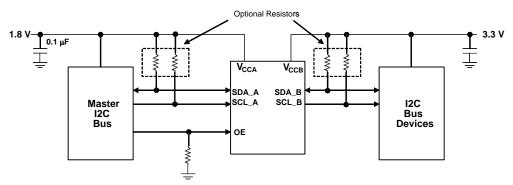
Design Notes: OE can be tied directly to 1.8 V (V<sub>CCA</sub>) to always be in ENABLE mode.
