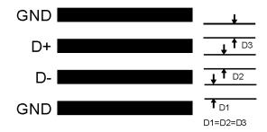
Figure 21. Ideal Diode Trace Layout
