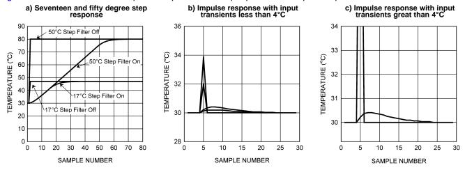
Figure 11. Filter Impulse and Step Response Curves
