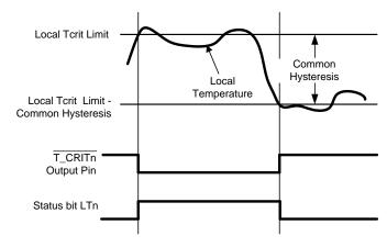
Figure 15. TCRIT response diagram (masking options not included)
