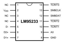
Figure 1. 14-Lead WSON - TOP VIEW See NHL0014B Package
