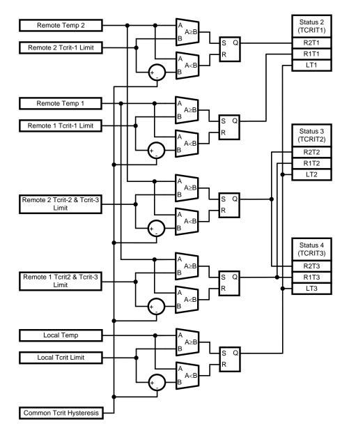
Figure 13. Temperature Comparison Logic and Status Register Simplified Diagram
