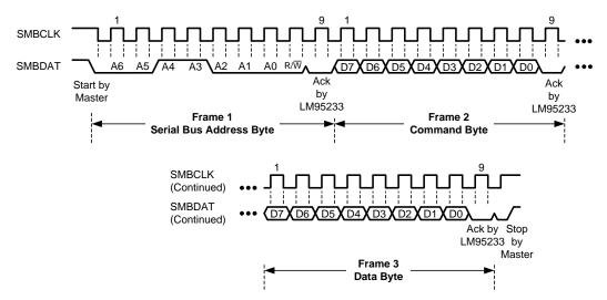
Figure 16. (a) Serial Bus Write to the internal Command Register followed by a the Data Byte
