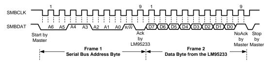
Figure 18. (c) Serial Bus Read from a Register with the Internal Command Register preset to desired value.
