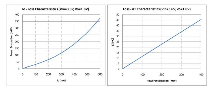
The output current of the device may need to be de-rated if it is operated in a high ambient temperature or in a continuous power delivering application. The amount of current de-rating is highly dependent on the environmental thermal conditions, i.e. PCB design, nearby components or effective air flows. Care should especially be taken in applications where the device temperature exceeds 85°C.
