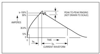
Figure 6b. Human Body Current Waveform
