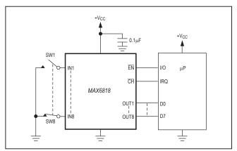
Figure 5. MAX6818 Typical μP Interfacing Circuit
