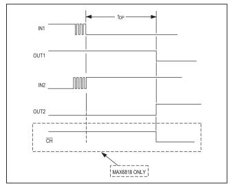
Figure 2. Input Characteristics
