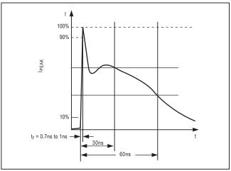
Figure 7b. IEC 1000-4-2 ESD Generator Current Waveform
