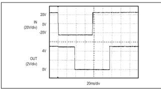
Figure 3. Switch Input ±25V Fault Tolerance
