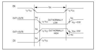
Figure 4. MAX6818 µP-Interface Timing Diagram
