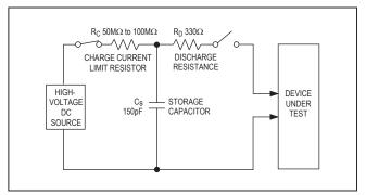
Figure 7a. IEC 1000-4-2 ESD Test Model
