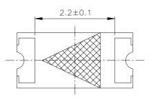
**Notes:** Tolerances Unless Dimension  $\pm 0.1$ mm , Angle $\pm 0.5^{\circ}$ , Unit = mm
