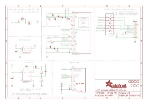
For the level shifter we use the CD74HC4050 (https://adafru.it/Ekk) which has a typical propagation delay of ~10ns
