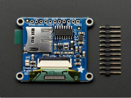
The breakout board comes fully assembled and tested. We include an optional strip of header pins to make it easier to use this display in a breadboard. The header can be installed in just a few minutes with your soldering iron:
