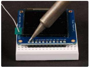
Position the display Place the display breakout on the header so that the short pins protrude through the holes.
