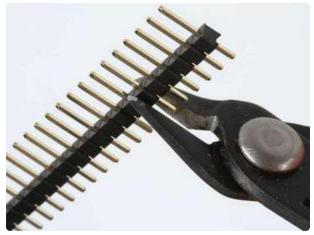
Prepare the header strip Cut the header to size and insert (long pins down) into a breadboard to stabilize for soldering.
