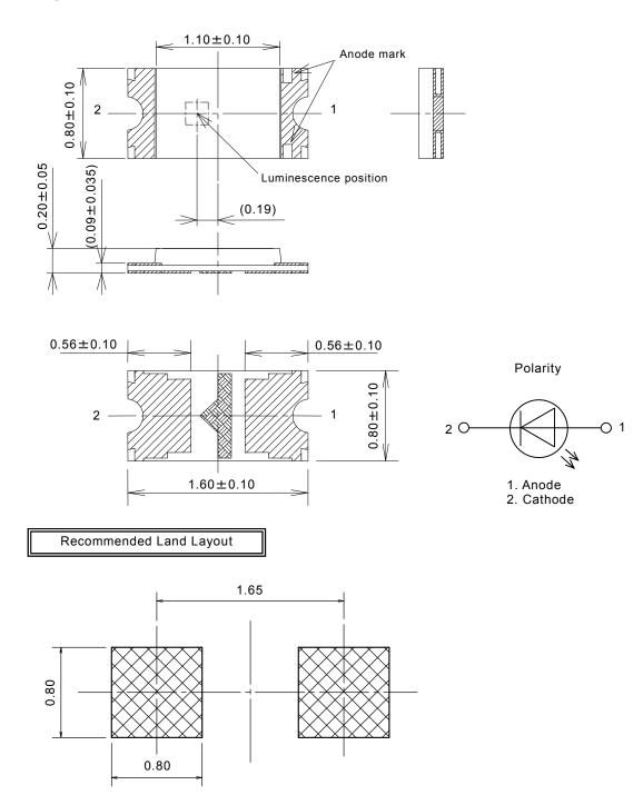
(Note1)Electrode projection is not included in the package dimensions. (Note2)About solder thickness, please examine the products yourself completely. (Recommended thickness : t=0.10 mm~0.15 mm)
