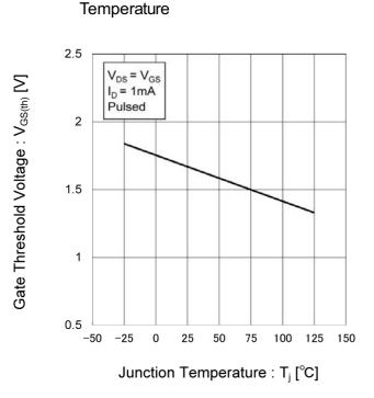
Fig.7 Gate Threshold Voltage vs. Junction
