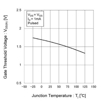
Fig.7 Gate Threshold Voltage vs. Junction Temperature
