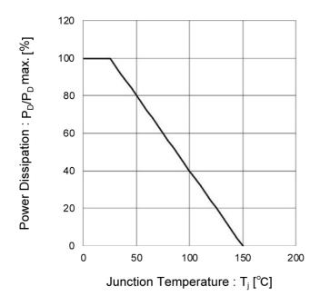
Fig.1 Power Dissipation Derating Curve
