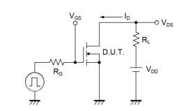
Fig.2-1 Gate Charge Measurement Circuit
