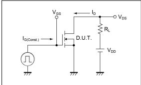
Fig.3-1 Avalanche Measurement Circuit
