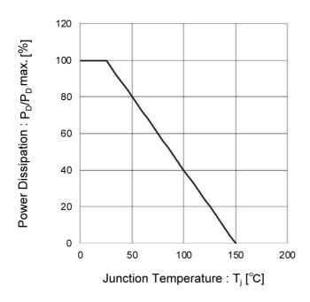
Fig.1 Power Dissipation Derating Curve
