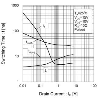
Fig.16 Switching Characteristics
