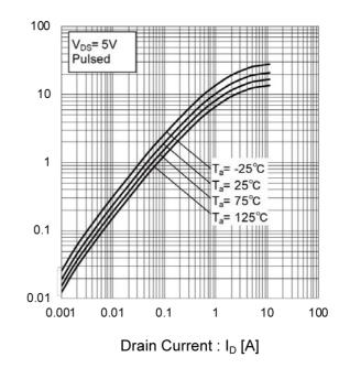
Fig.9 Drain Current Derating Curve
