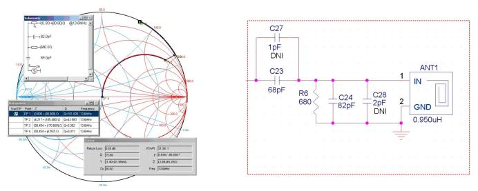
Figure 9. Smith Chart Simulation ( $R_{PAR} = 680 \Omega$ )
