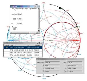
Figure 8. Smith Chart Simulation ( $R_{PAR} = 1.3 \text{ k}\Omega$ )
