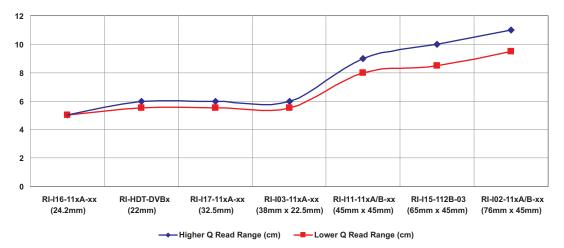
Figure 14. ISO15693 Transponder Read Ranges with TRF7960TB
