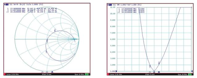
Figure 13. Lower Q Antenna Measurement Plots with Calculated Values (Q = ~10)
