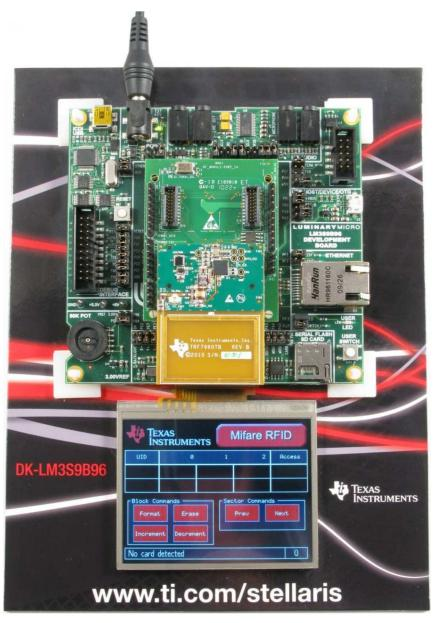
Figure 6. DK-LM3S9B96-EM2-TRF7960R Development Platform
