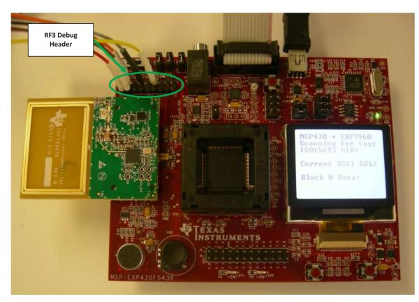
Figure 5. Firmware Development\Debug Setup for MSP-EXP430F5438 Experimenters Board
