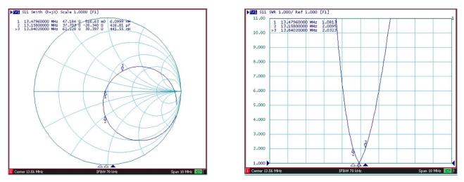
Figure 12. Higher Q Antenna Measurement Plots with Calculated Values (Q = ~20)
