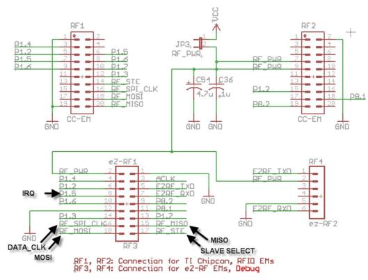
Figure 4. Debug Header (RF3) Logic Analyzer Connections for Monitoring SPI Communications Between MSP430F5438A and TRF796x on TRF7960TB Module
