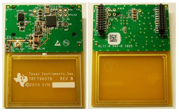
Figure 1. TRF7960TB Evaluation Module
