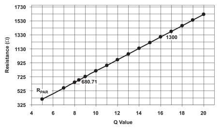
Figure 10. Theoretical Parallel Resistor Value for Desired Q
