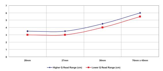
Figure 15. ISO14443A Transponder Read Ranges with TRF7960TB
