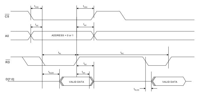
Figure 3. Parallel Interface Read Timing
