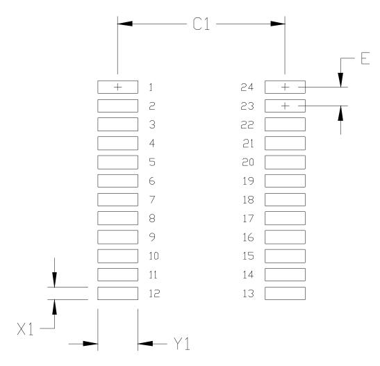
Figure 22. 24-Pin TSSOP Land Pattern Diagram
