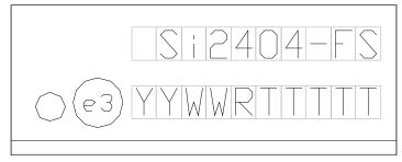
Figure 18. Si2404-D-FS Top Marking
