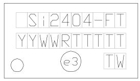
Figure 17. Si2404-D-FT Top Marking
