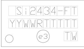
Figure 13. Si2434-D-FT Top Marking
