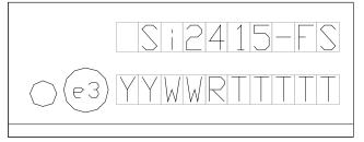
Figure 16. Si2415-D-FS Top Marking
