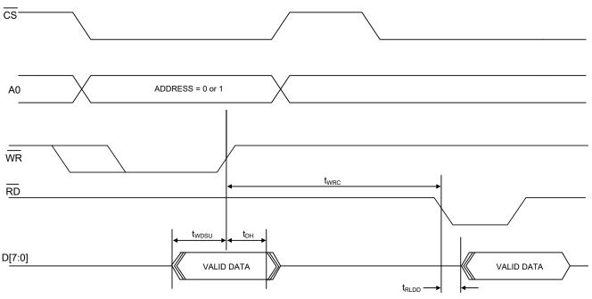
Figure 5. Parallel Interface Write Followed by Read Timing
