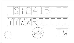
Figure 15. Si2415-D-FT Top Marking
