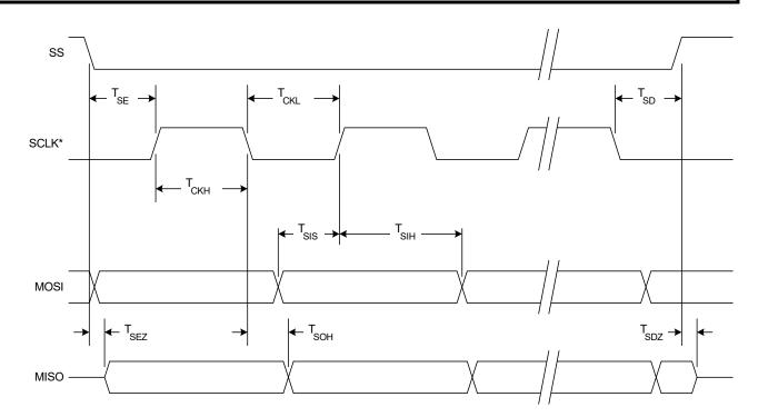
Figure 2. SPI Slave Timing
