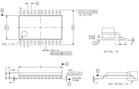
Figure 21. 24-Pin Thin Shrink Small Outline Package (TSSOP)
