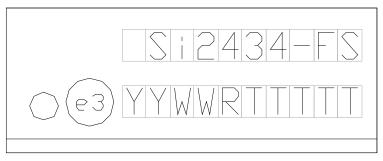
Figure 14. Si2434-D-FS Top Marking
