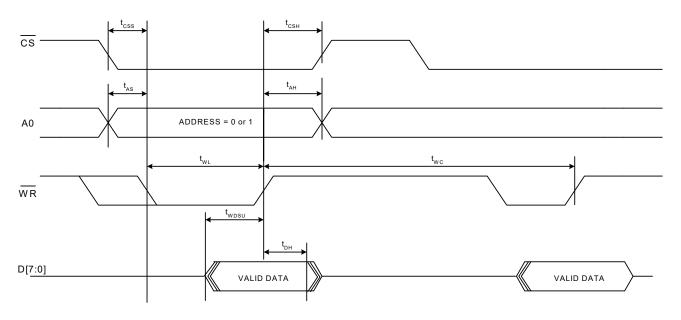
Figure 4. Parallel Interface Write Timing
