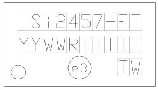
Figure 11. Si2457-D-FT Top Marking
