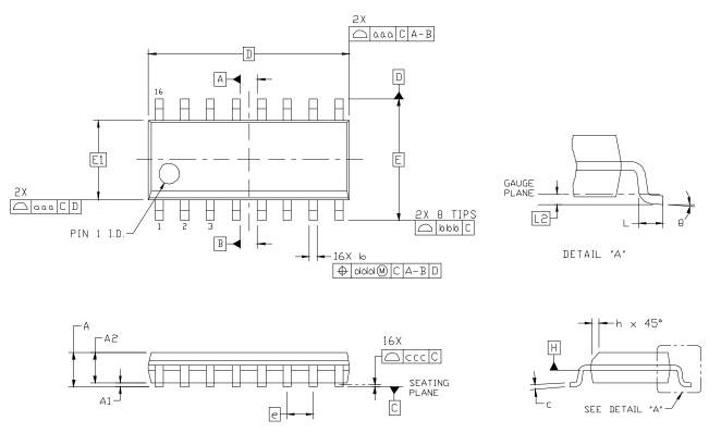
Figure 23. 16-Pin Small Outline Integrated Circuit (SOIC) Package
