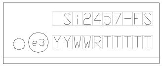
Figure 12. Si2457-D-FS Top Marking
