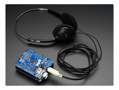
Bend all audio files to your will with the Adafruit Music Maker shield for Arduino! This powerful shield features the VS1053, an encoding/decoding (codec) chip that can decode a wide variety of audio formats such as MP3, AAC, Ogg Vorbis, WMA, MIDI, FLAC, WAV (PCM and ADPCM). It can also be used to record audio in both PCM (WAV) and compressed Ogg Vorbis. You can do all sorts of stuff with the audio as well such as adjusting bass, treble, and volume digitally.
