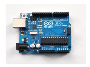
Begin by breaking the 36-pin male header into four pieces: one 10-pin, two 8-pin and one 6-pin. Stick the header into the Arduino sockets with the long pins down.
