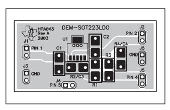
Figure 3. PCB Layout – Top Assembly
