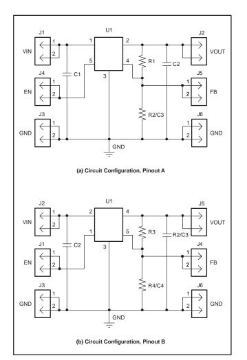
Figure 2. Example Board Configurations for Evaluating SOT223 LDOs
