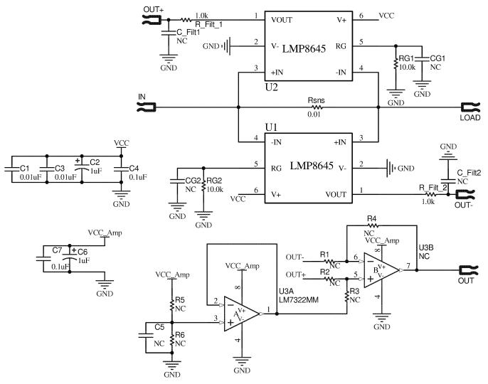
Figure 2. Schematic Diagram
