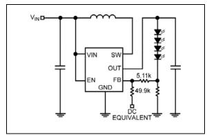
FIGURE 4-2: Continuous Dimming.
