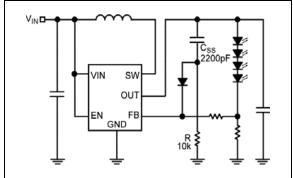
FIGURE 4-4: Soft-Start Circuit.
