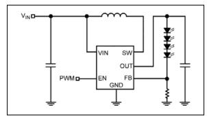
FIGURE 4-1: PWM Dimming Method.
