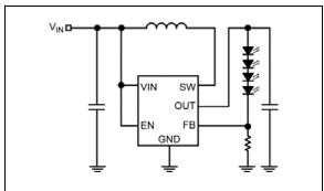
FIGURE 4-3: DFN Package OVP Circuit.
