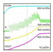
Figure 9. Startup Behavior of Current Limit Based Softstart.
