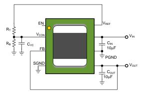
Figure 12. Typical Application Circuit
