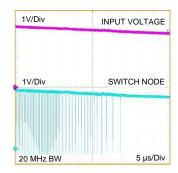
Figure 11. High Duty Cycle Operation and Switching Frequency Reduction
