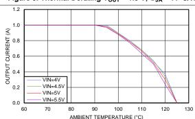
Figure 4. Thermal Derating  $V_{OUT}$  = 2.5 V,  $\Theta_{JA}$  = 77°C/W
