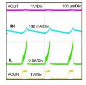
Figure 10. Hiccup Behavior with Persistent Output Short Circuit.
