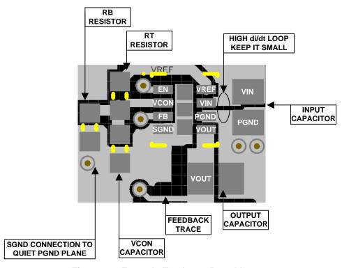
Figure 37. Example Top Layer Board Layout
