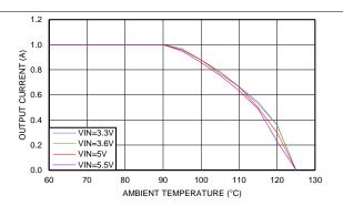
Figure 3. Thermal Derating  $V_{OUT}$  = 1.8 V,  $\Theta_{JA}$  = 77°C/W
