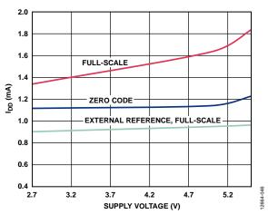
Figure 37. IDD vs. Supply Voltage
