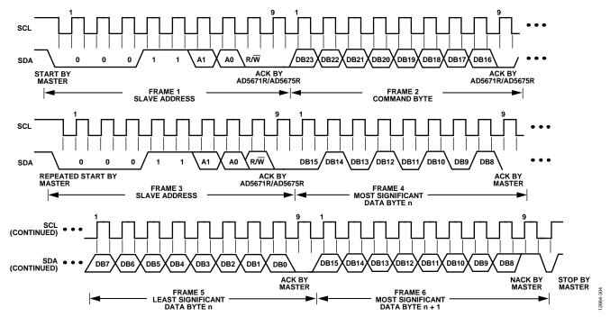
Figure 60. I<sup>2</sup>C Read Operation
