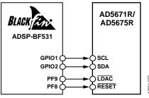
Figure 67. AD5671R/AD5675R to ADSP-BF531 Interface
