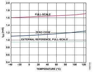
Figure 36. IDD vs. Temperature
