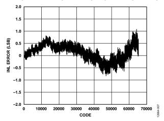
Figure 6. AD5675R INL Error vs. Code
