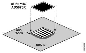
Figure 68. Pad Connection to Board
