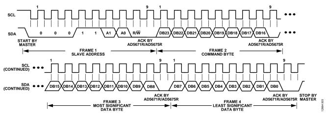
Figure 59. I<sup>2</sup>C Write Operation
