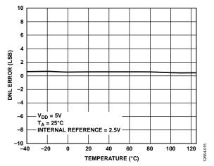
Figure 14. AD5675R DNL Error vs. Temperature
