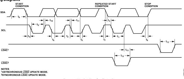
Figure 2. 2-Wire Serial Interface Timing Diagram
