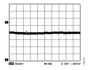
Figure 45. 0.1 Hz to 10 Hz Output Noise Plot
