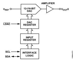
Figure 62. Simplified Diagram of Input Loading Circuitry for a Single DAC
