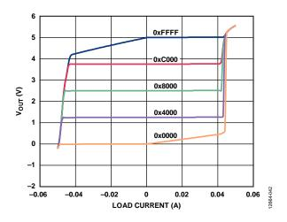
Figure 33. Source and Sink Capability at 5 V
