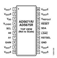
Figure 4. TSSOP Pin Configuration
