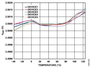
Figure 52. V<sub>REF</sub> vs. Temperature (B Grade)
