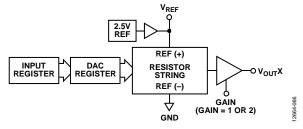
Figure 55. Single DAC Channel Architecture Block Diagram
