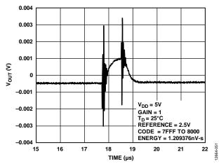
Figure 42. Digital-to-Analog Glitch Impulse
