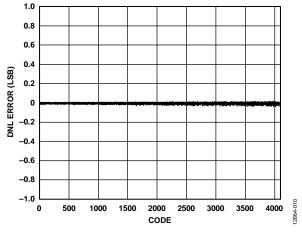
Figure 9. AD5671R DNL Error vs. Code
