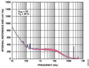
Figure 50. Internal Reference NSD vs. Frequency
