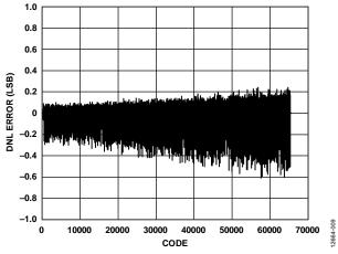
Figure 8. AD5675R DNL Error vs. Code
