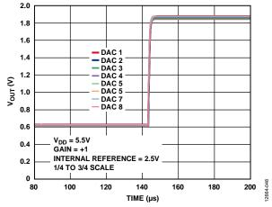
Figure 39. Full-Scale Settling Time
