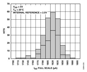
Figure 31. IDD Histogram with Internal Reference
