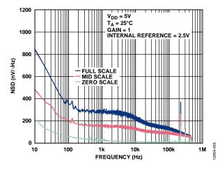
Figure 46. Noise Spectral Density (NSD)
