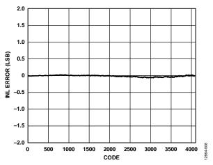
Figure 7. AD5671R INL Error vs. Code
