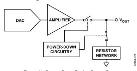
Figure 61. Output Stage During Power-Down
