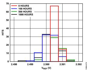
Figure 64. Reference Drift Through to 1000 Hours
