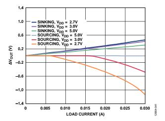
Figure 32. Output Voltage Change (ΔV<sub>ΟUT</sub>) vs. Load Current
