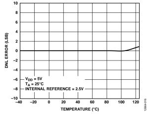
Figure 15. AD5671R DNL Error vs. Temperature
