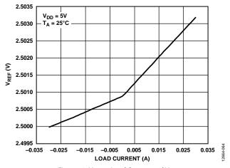
Figure 53.  $V_{REF}$  vs. Load Current and  $V_{DD}$
