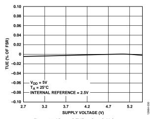
Figure 22. AD5671R TUE vs. Supply Voltage
