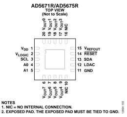
Figure 5. LFCSP Pin Configuration
