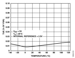
Figure 17. AD5671R TUE vs. Temperature
