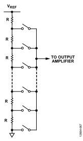
Figure 56. Resistor String Structure
