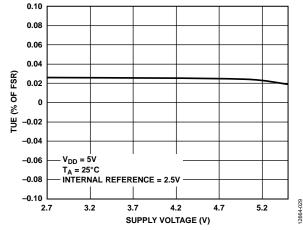
Figure 21. AD5675R TUE vs. Supply Voltage
