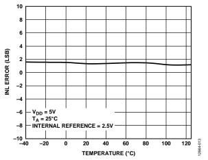
Figure 12. AD5675R INL Error vs. Temperature
