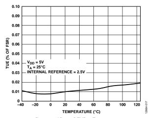
Figure 16. AD5675R TUE vs. Temperature
