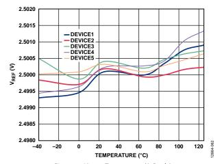
Figure 51. V<sub>REF</sub> vs. Temperature (A Grade)
