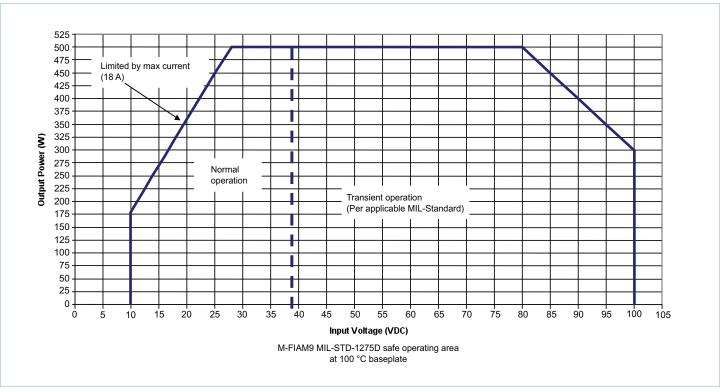
Figure 6 — M-FIAM 9 transient safe operating area at 100°C baseplate
