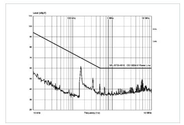
**Figure 2** — Conducted noise: M-FIAM9 and model V28A12M200B DC-DC converter operating at 28V<sub>DC</sub>, 200W
