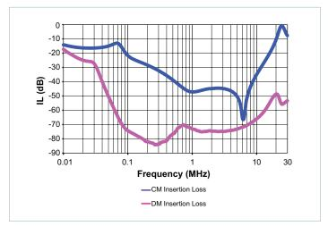
Figure 4 — M-FIAM9 insertion loss
