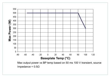
Figure 5 — Temperature de-rating
