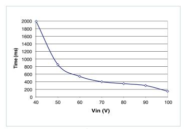
Figure 3 — Shut-down time of M-FIAM9 vs. overvoltage
