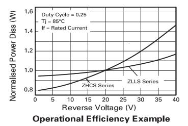
The operational efficiency chart indicates the beneficial use of the ZLLS series diodes in applications requiring higher voltage, higher temperature operation. Circuits requiring low voltage low temperature operation will benefit from using Zetex low VF ZHCS series diodes.
