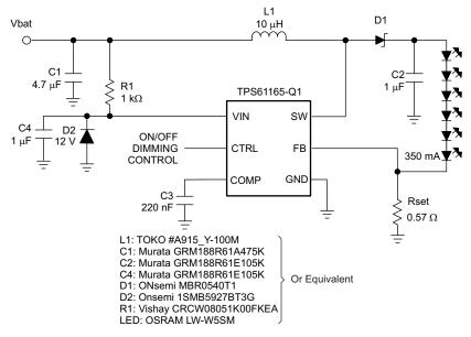
Figure 15. Drive Six High-Brightness LEDs
