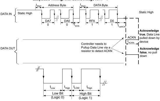
Figure 14. EasyScale— Bit Coding
