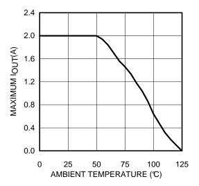
$\theta_{JA} = 40$  °C/W,  $V_{OUT} = 3.3$  V,  $f_{SW} = 500$  kHz (tested on the evaluation board)
