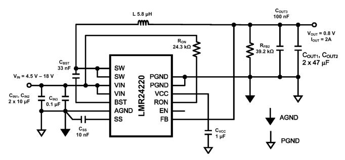
Figure 26. Typical Application Schematic For  $V_{OUT} = 0.8 \text{ V}$
