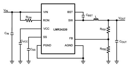
Figure 20. Typical Application Schematic
