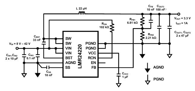
Figure 25. Typical Application Schematic For  $V_{OUT} = 3.3 \text{ V}$
