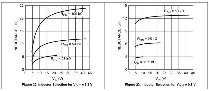
Figure 22 and Figure 23 show curves on inductor selection for various  $V_{OUT}$  and  $R_{ON}$ . For small  $R_{ON}$ , according to Equation 10,  $V_{IN}$  is limited. Some curves are therefore limited as shown in the figures.
