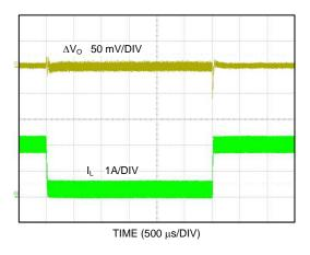
$V_{OUT}$  = 3.3 V, 0.2 A to 2 A Load
