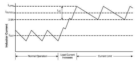
Figure 18. Inductor Current - Current Limit Operation
