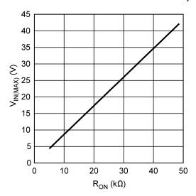
Figure 21. Maximum V<sub>IN</sub> for Selected R<sub>ON</sub>
