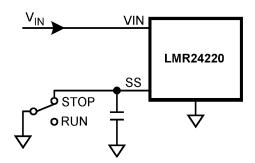
Figure 19. Alternate Shutdown Implementation
