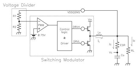
Figure 3. Linearizing the Modulator
