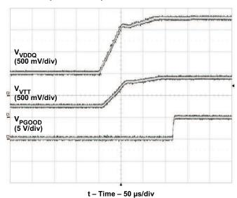
Figure 31. Pre-Biased Start-Up: VDDQ, VTT, and PGOOD
