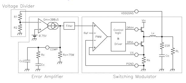
Figure 2. Linearizing the Modulator
