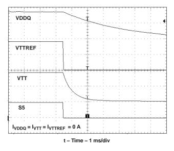
Figure 32. Soft-Stop Waveforms Non-Tracking Discharge
