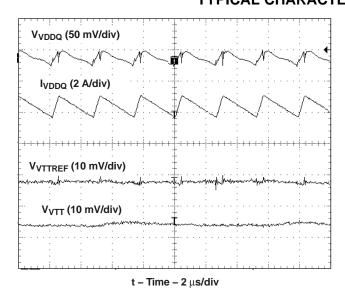
Figure 26. Ripple Waveforms - Heavy Load Condition
