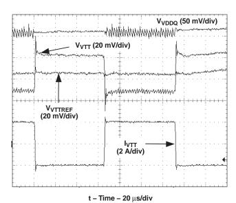
Figure 28. VTT Load Transient Response
