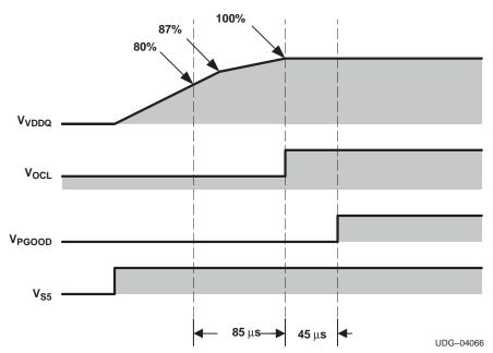
Figure 1. VDDQ Soft-Start and Powergood Timing
