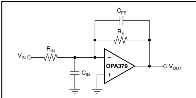
Figure 22. Improving Stability for Large  $R_F$  and  $R_{IN}$
