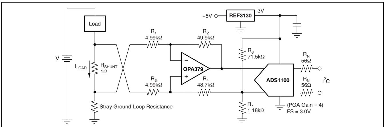
NOTE: 1% resistors provide adequate common-mode rejection at small ground-loop errors.
