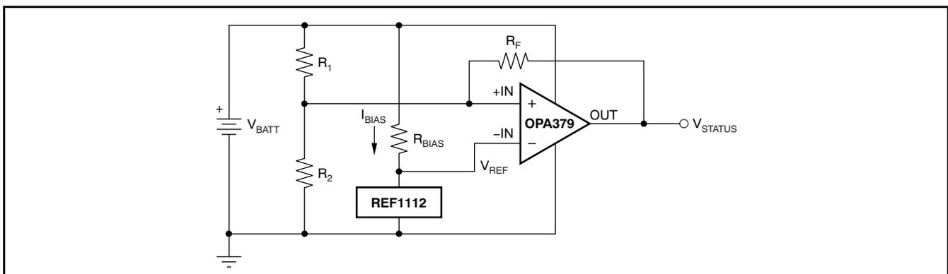
Figure 23. Battery Monitor
