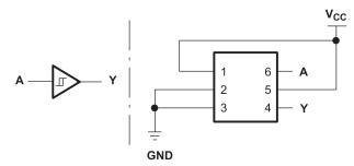
Figure 6. Noninverted Buffer
