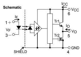
0.1  $\mu\text{F}$  bypass capacitor must be connected between pin 6 and 4.
