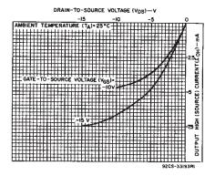
Fig. 13 — Minimum p-channel output high (source) current characteristics.
