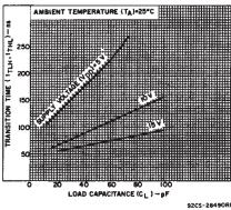
Fig.6 - Typical transition time vs. load capacitance.
