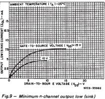
Fig.9 — Minimum n-channel output low (sink) current characteristics.
