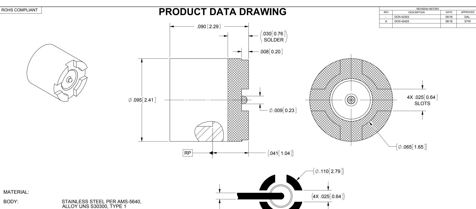
PIN: **KOVAR PER ASTM-F15**
