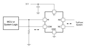
Figure 24. System Schematic for TS5A3160
