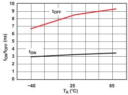
Figure 25.  $t_{ON}$  and  $t_{OFF}$  vs Temperature (V<sub>+</sub> = 5 V)
