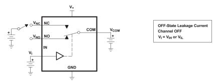
$\textbf{Figure 14. OFF-State Leakage Current (I}_{NC(OFF)}, I_{NO(OFF)}, I_{COM(OFF)}, I_{NC(PWROFF)}, I_{NO(PWROFF)}, I_{COM(PWROFF)})\\$
