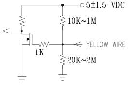
14–1. THE FAN SPEED WILL DEFAULT TO MAXIMUM WHEN THE SPEED CONTROLL INPUT IS LEFT UNCONNECTED.
