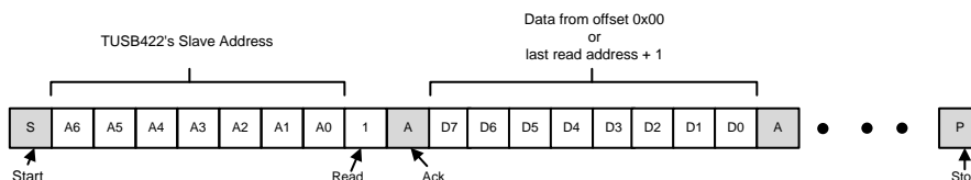
Figure 7. I2C Read Without Repeated Start
