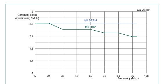
Conditions:  $V_{DD}$  = 3.3 V;  $T_{amb}$  = 25 °C; active mode; all peripherals except one UART; BOD disabled; SRAM0 and SRAM1 powered, SRAM2 powered down. See the FLASHCFG register in the LPC5410x User Manual for system clock flash access time settings. Measured with Keil uVision 5.12. Optimization level 3, optimized for time on.
