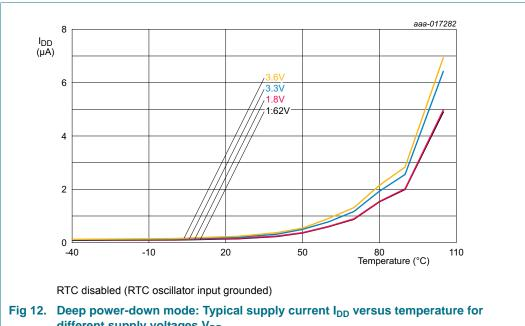
different supply voltages V<sub>DD</sub>
