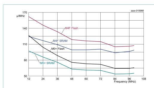
Conditions:  $V_{DD}$  = 3.3 V;  $T_{amb}$  = 25 °C; active mode; all peripherals disabled; BOD disabled; Prefetch disabled in FLASHCFG register. System clock flash access time set by power API. SRAM0 powered, SRAM1 and SRAM2 powered down. Measured with Keil uVision 5.12. Optimization level 0, optimized for time off.
