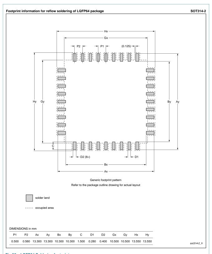
Fig 36. LQFP64 Soldering footprint
