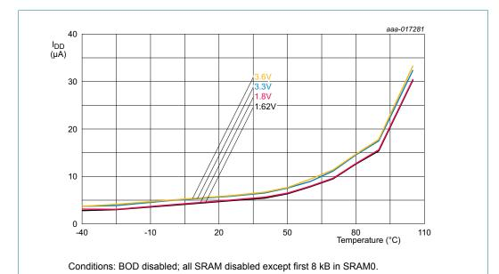
Fig 11. Power down mode: Typical supply current  $I_{DD}$  versus temperature for different supply voltages  $V_{DD}$
