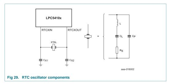
For best results, it is very critical to select a matching crystal for the on-chip oscillator. Load capacitance ( $C_L$ ), series resistance ( $R_S$ ), and drive level ( $D_L$ ) are important parameters to consider while choosing the crystal. After selecting the proper crystal, the external load capacitor  $C_{X1}$  and  $C_{X2}$  values can also be generally determined by the following expression:
