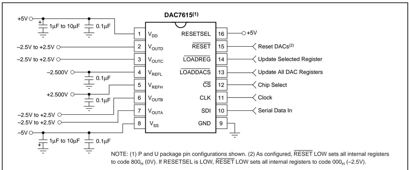
FIGURE 2. Basic Dual-Supply Operation of the DAC7615.
