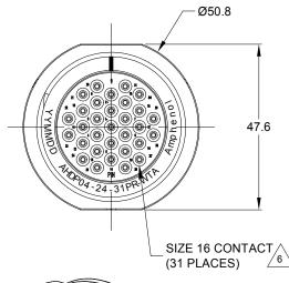
RECEP.,24-31 POS, PIN CONT., REDUCED DIA. SEAL, AHDP
