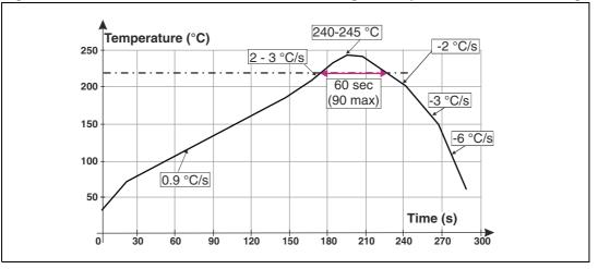
Figure 12. ST ECOPACK<sup>®</sup> recommended soldering reflow profile for PCB mounting
