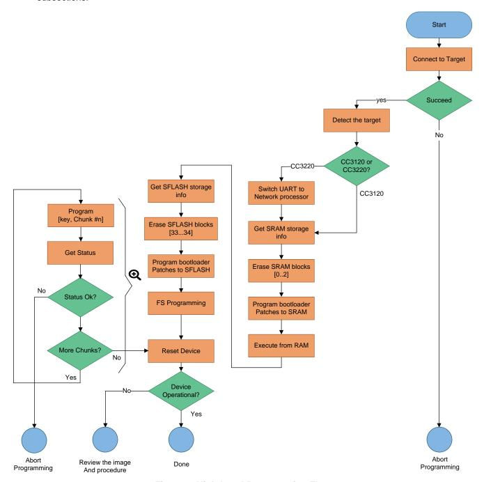
Figure 2. High-Level Programming Flow
