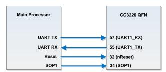
Figure 1. CC3120 and CC3220 QFN Programming Setup
