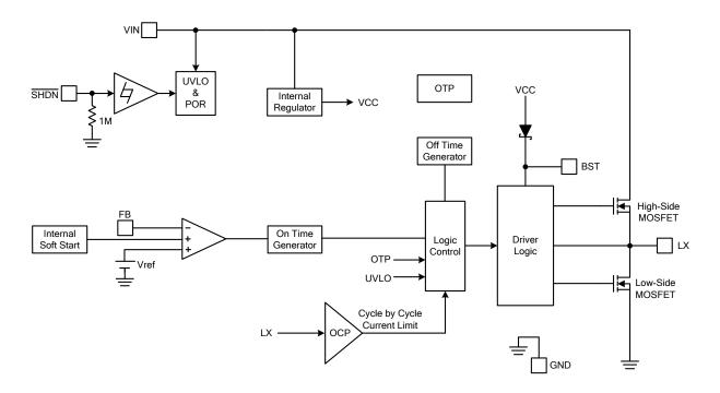
Figure 3. Block Diagram of FR9205F
