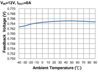
Figure 9. Feedback voltage vs. Temperature
