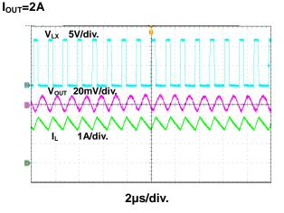
Figure 11. Steady State Waveform
