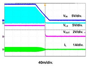
Figure 14. Shutdown Through Power Supply Waveform
