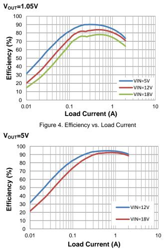
Figure 6. Efficiency vs. Load Current
