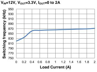
Figure 8. Switch Frequency vs. Load Current
