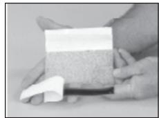
**3.5 Position Mold Body Around Splice.** Center mold body along connector. Wrap mold body around connection.
