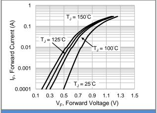
Fig.4 Typical Forward Characteristics
