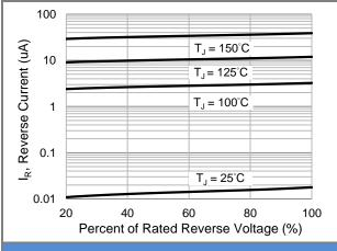
Fig.3 Typical Reverse Characteristics
