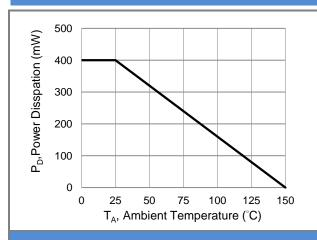
**Fig.1 Power Derating Curve**
