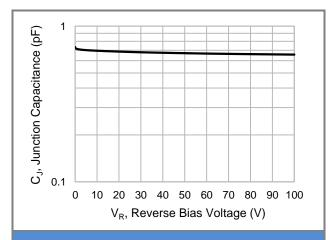
**Fig.2 Typical Junction Capacitance**
