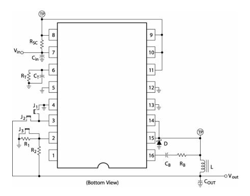
For Vout = 5.0 V: J1=open, J2=closed, and J3=closed For Vout = 3.3 V: J1=closed, J2=open, and J3=open
